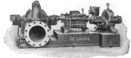
De Laval Centrifugal Circulating Pump driven by geared steam turbine, 6500 g.p.m., 25 feet head.
