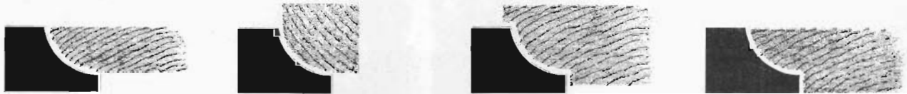
FIG. 2. ILLUSTRATES TYPICAL CUTTER (No. 422) USED FOR MORE THAN ONE CUT.
