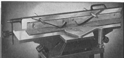
Spring Hold-Downs for safe feeding of short or thin materials. Keeps hands away from cutterhead. Also holds long lumber down while you feed from a position several feet distant from machine. Convenient "Hand-Hold" on fence facilitates easy tilting or lateral movements. Fence has 4 holes for attaching wood facings.
