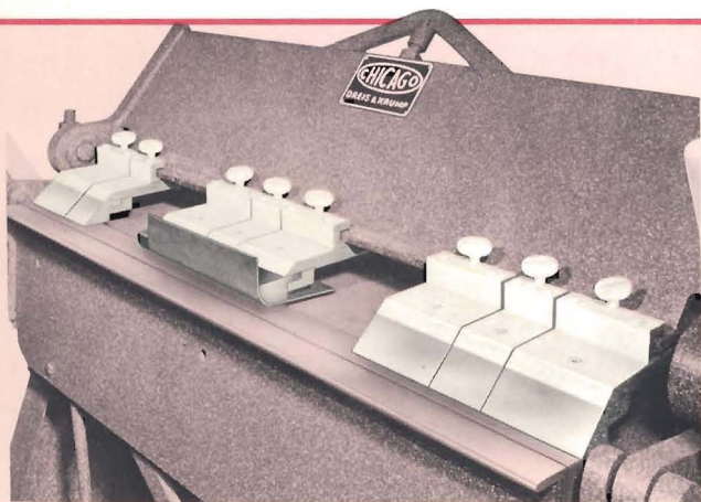
Fig. 14 —Radius nose bar used in lieu of straight bending fingers for forming contemporary furniture, cabinets.
