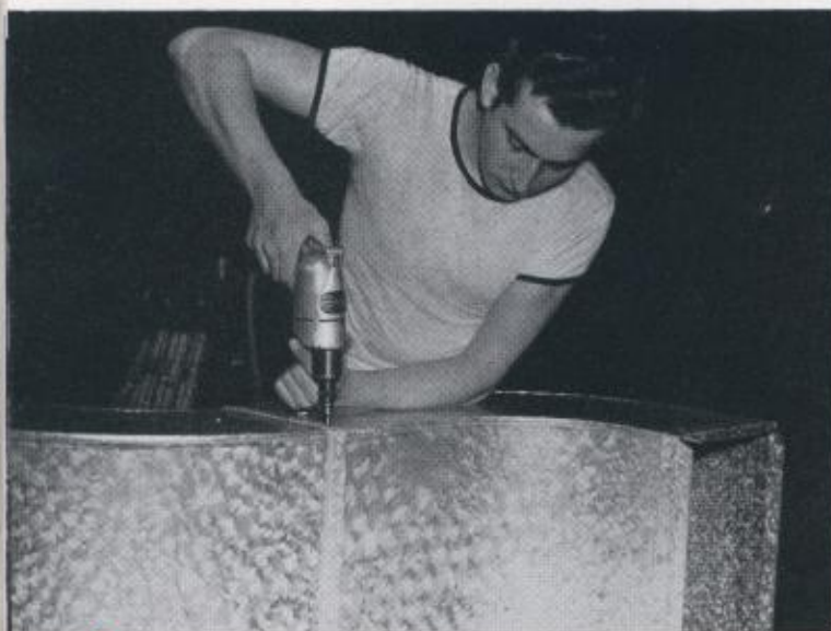
↑ Fabrication of air conditioning ducts requires hundreds of sheet metal screws. No. 8 Positive Clutch Scrugun steps up production.
