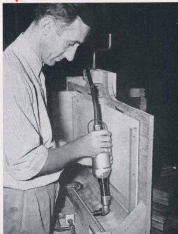
↓ Radio cabinet assembly. No. 8-90° Center-Drive Scrugun easily handles close-corner wood screw driving.
