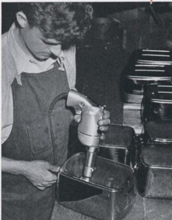
No. 22 Positive Clutch Driver (with reversing switch) attaching lashing lugs to truck body. ↑
