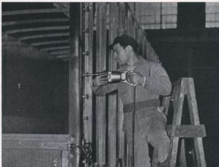
No. 22 Positive Clutch Driver (with reversing switch) attaching lashing lugs to truck body. ↑
