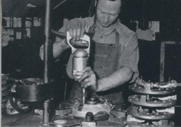
↑ No. 12 Positive Clutch Driver tightens lock nuts on automobile clutch assembly. Tool is suspended for faster work—less fatigue.
