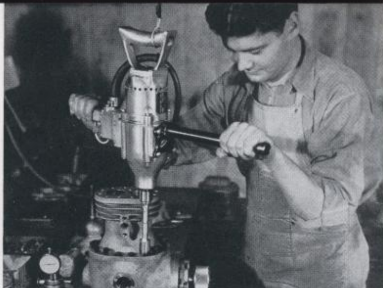
Absolute tightness and uniformity are essential in compressor head assembly. High Cycle Driver does the job. ↑
