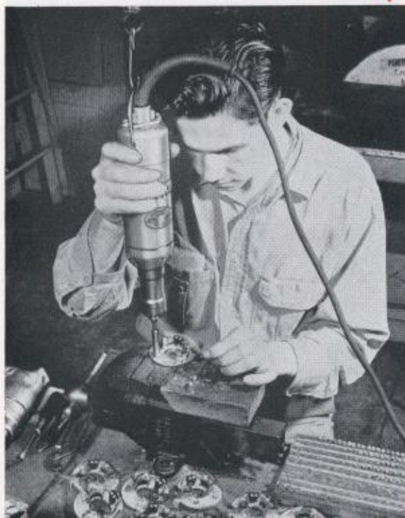
No. 8 Adjustable Clutch Center-Driver Scrugun provides the "watch-maker" accuracy required in assembling distributor parts. ↓
