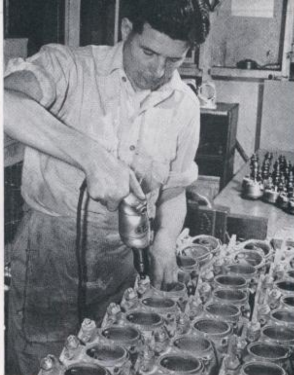
↑ For delicate carburetor assembly, the No. 8 Adjustable Clutch Scrugun provides exactly correct driving torque.
