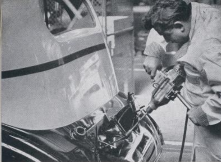
↑ High Cycle Driver assembling tire carrier on automobile assembly line.
