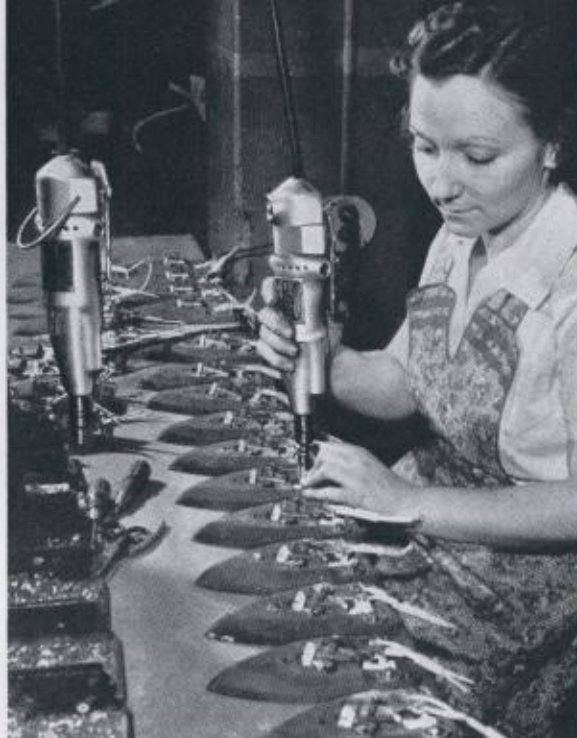
↑ A pair of Torsimeters on electric iron assembly. One equipped with socket-wrench and reversing switch; the other with screw-bit; both have paddle switches.
