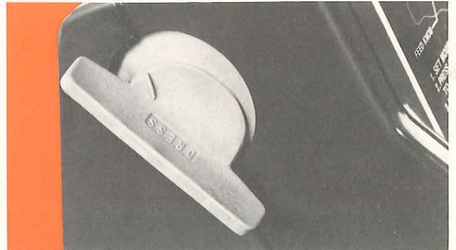
1. Line up mark on dress knob with parting line of housing. Position swinghead close to the eyeshield.
