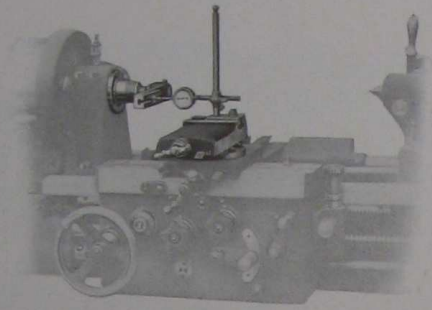
Testing cross slide alignment (Fig. No. 1)
