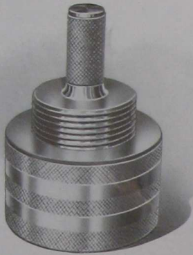
Hardened and lapped master for spindle noses and face plates (Fig. No. 1)
