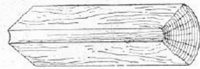
Bolt cut to uniform length on Bolt Equalizer ready for cylinder stave sawing machine.
