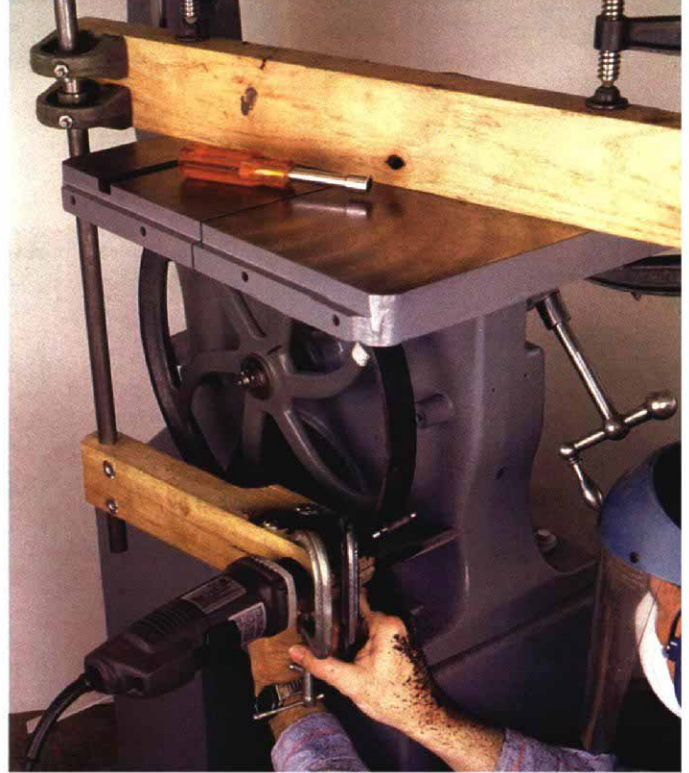
pivot shaft extending, up for working on the top wheel (left) or down for the bottom wheel (right). Each tire is trimmed twice at a slight angle from each outer edge to form a V-shaped crown.
