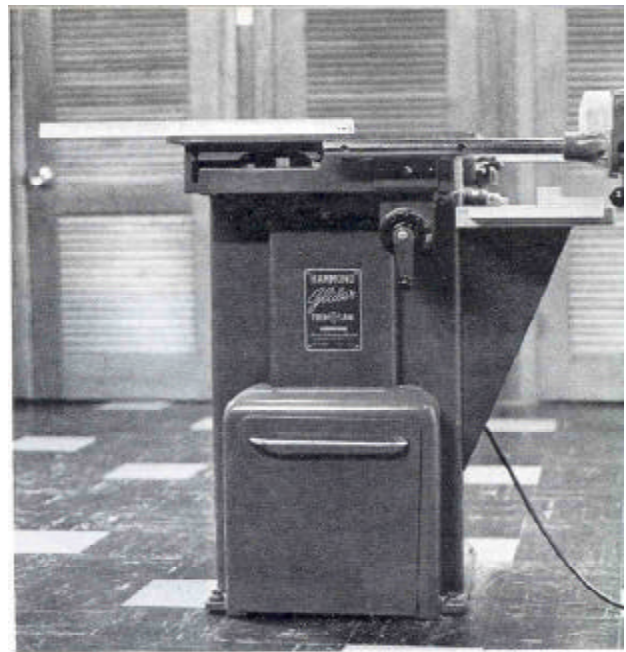
The Hammond Trim-O-Saw, originally used for cutting lead type in newspaper composing rooms, becomes an accurate woodworking machine for mortising and precise cutting.
