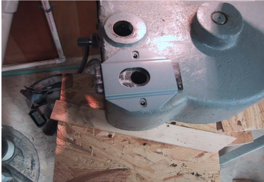
Figure 7 – completed tapped holes (note that the retainer is erroneously upside-down in this photo – the shaft hole should be toward the bottom of the gearbox)
