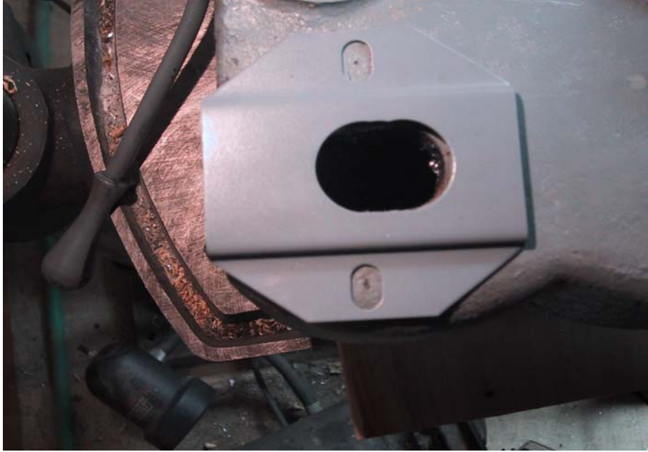
Figure 5 – dimples placed, ready for drilling
