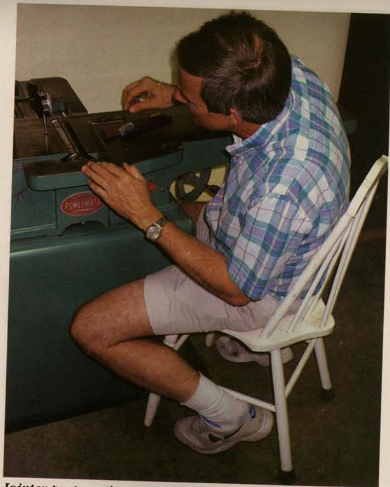
Jointer preparation involves clearing the area and getting comfortable. Tools the author has gathered for the job include a dial indicator, a toothbrush for cleaning parts and an extension pipe to apply torque to his custom-ground setscrew wrench.
