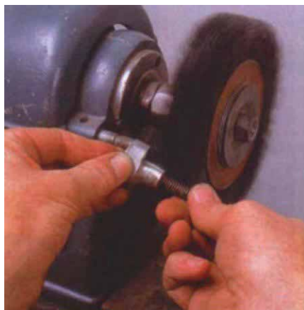
A fine-wire brush mounted on the author's wood lathe quickly and efficiently cleans away dirt, dried grease and even light rust. The wheel also imparts a slight polish, so Vaughan runs all fastener heads under the wheel for a few seconds.
