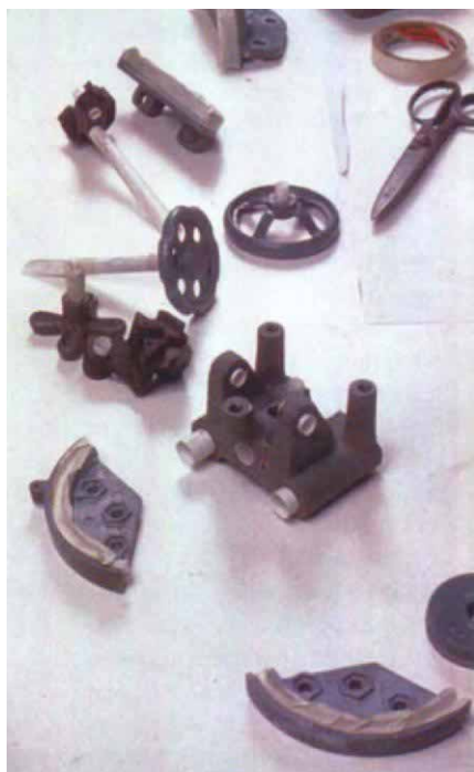
Masking all parts ensures a clean, crisp, professional-looking paint job. A good way of masking holes is to wrap a piece of paper tightly around a dowel and then to release it inside the hole. The paper will expand to fit. To avoid a messy cleanup later, remove all the masking tape as soon as the paint is dry enough to touch.
