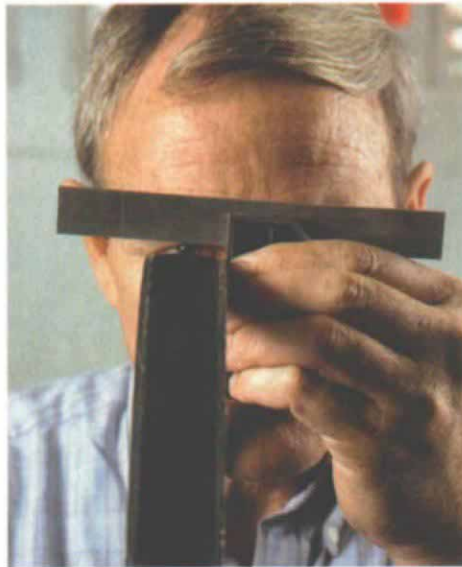
Tires need a crowned surface. A smooth tire with a slightly crowned surface, like this one, will make a bandsaw track accurately and run smoothly.
