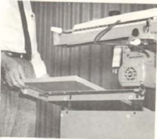
9. Fit table top assembly to machine frame so that the four drilled holes (circled in white) match.
