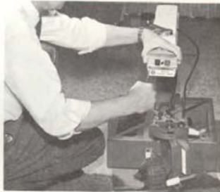
6. Remove two screws from arm endcap, wipe arm tracks with clean cloth.
