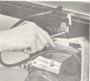
8. Loosen pointer screws, adjust both pointers to up-right position and tighten screws.
