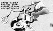
TO TIGHTEN OR LOOSEN NUT, WRENCH UNDER TABLE ENGAGES FLAT SPOT ON SPINDLE
